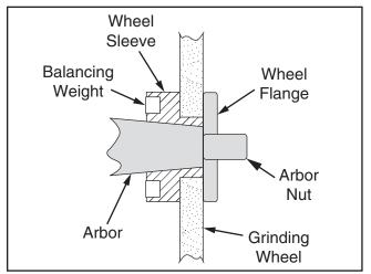
Figure 33. Wheel assembly components.
